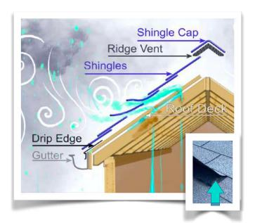
inherently waterproof? They're designed to shed water due to their overlapping fish-scale arrangement. While the sticky asphalt helps them adhere and usually holds up, during powerful storms with upward water pressure, a waterproof underlayment like synthetic felt or ice guard becomes crucial. This prevents potential leaks, highlighting the significance of proper underlayment in extreme weather."
