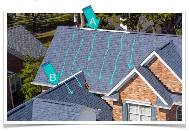
To protect the water from accessing the leak area, your tarp needs to overlap both Ridge **A** and Ridge **B**.
