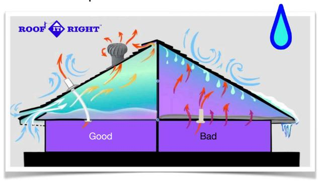
Another common mistake is leading the moisture or heated air from a bathroom or another exhaust pipe into the attic space instead of all the way to the roof. In general, condensation accumulates when there is either too much warm air circulating upwards from living spaces or when there is inadequate roofing ventilation or insulation.
